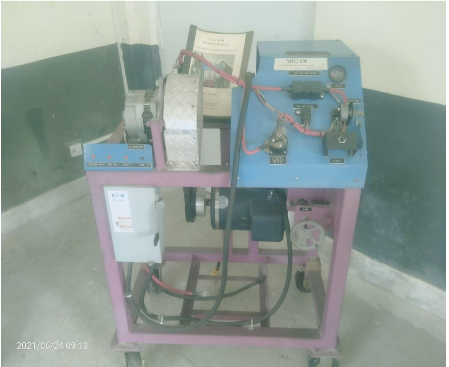
Mack Truck Charging /Cranking Trainer
