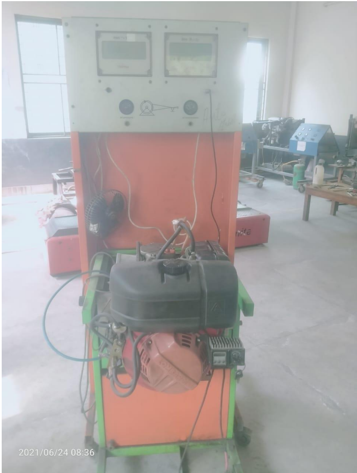
Small Engine Dynamometer (for Engines) with Horizontal and Vertical Operation Position
